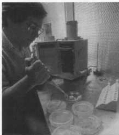
At the Plant Gene Expression Center, Albany, CA, a microbiologist uses a pipette to place the gene and tungsten mixture that will be blasted into plant cells within the gene gun.
