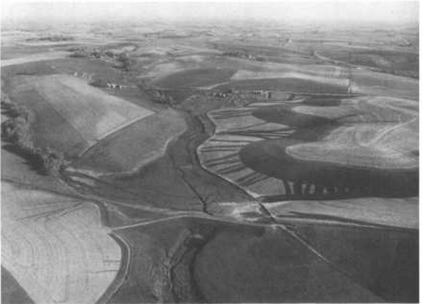
There once was a reservoir in the center of this area. Land adjacent to the reservoir was converted from pasture to row crops, and within 5 years the structure completely silted in. (Tim McCabe, SCS, IA-2873)
