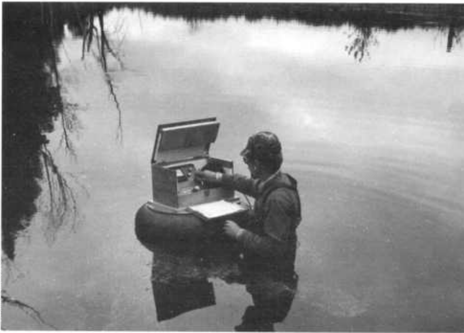
Maintaining high-quality water for fish and wildlife is an important aspect of forest management. North Central Forest Experiment Station technician measures dissolved oxygen and temperature in an experimental wildlife impoundment.
