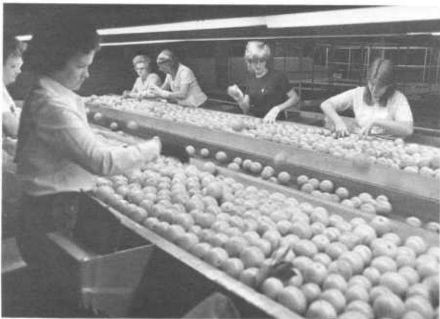
Farmers value co-ops as an assured market outlet. Workers in this Haines City (Fla.) Citrus Growers Association packing plant examine every orange and reject those that do not make U.S. Grade No. 1. Losers go to the juice plant.
