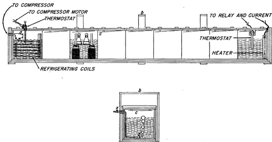
FIGURE 1.—Sectional views of water-bath apparatus used in making temperature studies.
