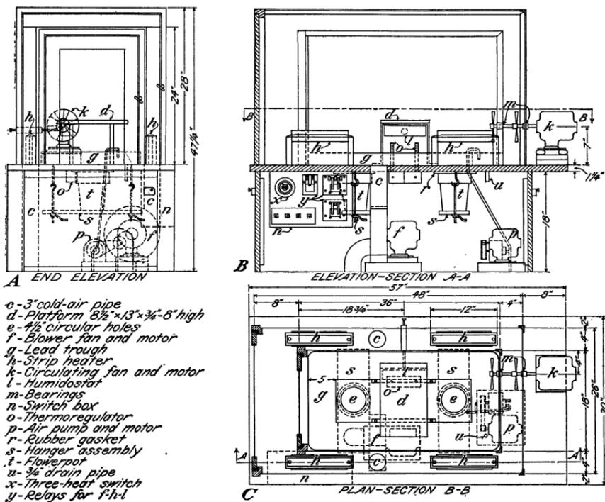
FIGURE 2.—Details of construction of the humidity- and temperature-control cabinet.
