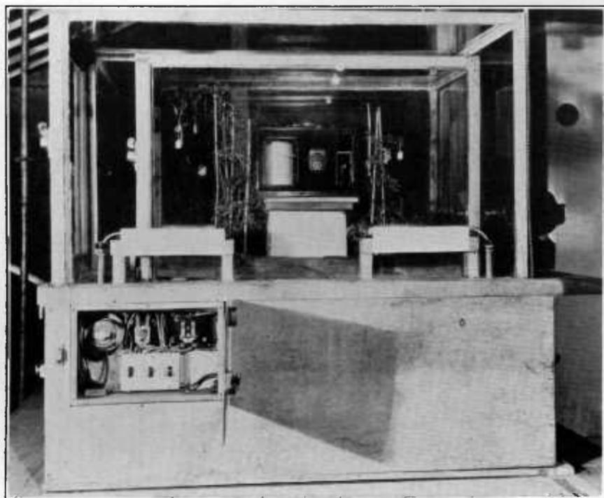
FIGURE 1.—Humidity- and temperature-control cabinet.
