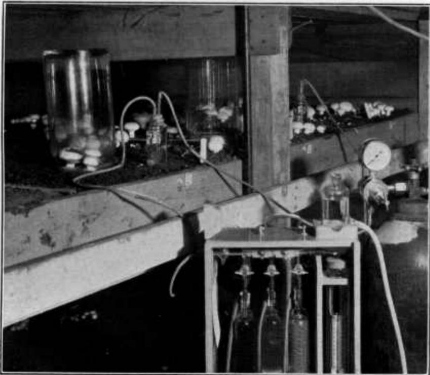
FIGURE 1.—Apparatus used for altering and testing the carbon dioxide and oxygen content of air surrounding growing mushrooms.
