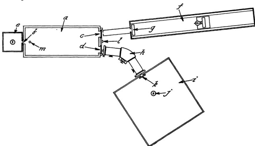
FIGURE 1.—Diagram (plan) of apparatus used to ascertain the intensity of white light necessary to produce stimulative effects upon bees equal to those of the light from selected lines of the mercury-vapor spectrum. (For explanation, see text.)
