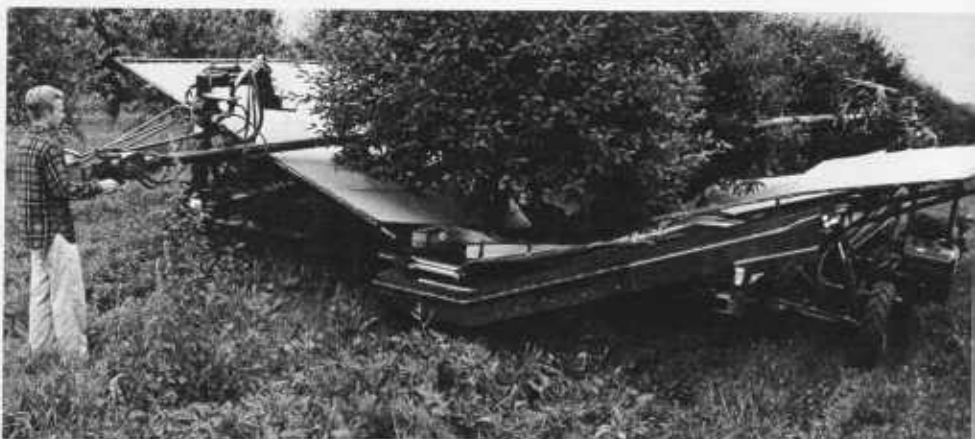
Cherry harvester, top , is positioned beneath tree. It has two hydraulic shakers and a catching frame. Elevator takes fallen cherries to cold water tank. In processing plant, below , each of these eight electric sorters can handle up to 2,800 pounds of cherries an hour.
