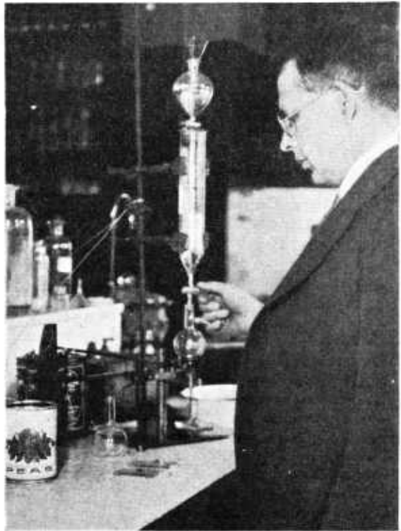
FIGURE 138.—V. B. Bonney using apparatus designed by him and other chemists to test the tenderness of canned peas
