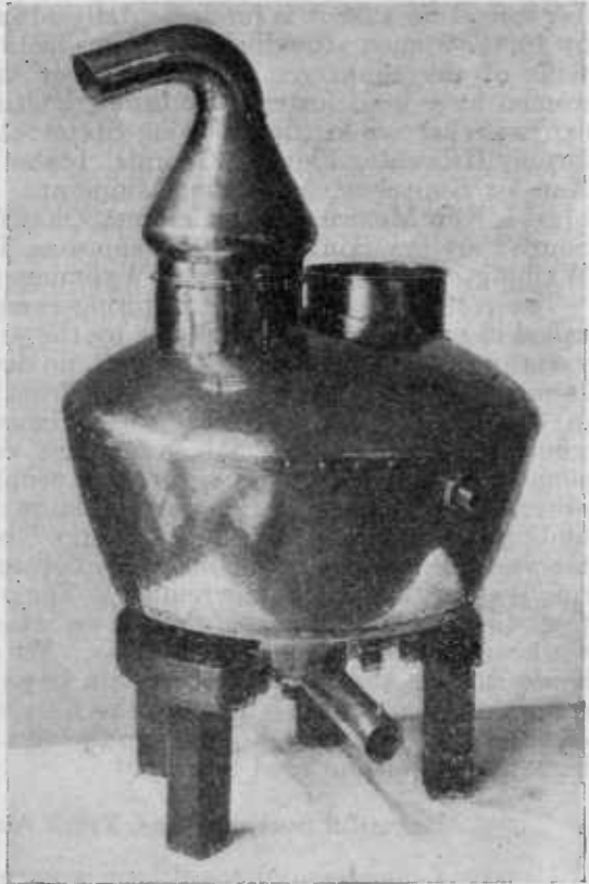
FIG. 272.—Model of the steam turpentine still designed by the United States Department of Agriculture
