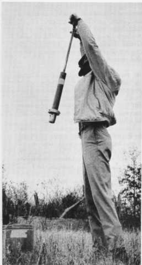
Hand-operated corer is used to collect soil samples in pesticide monitoring study.
