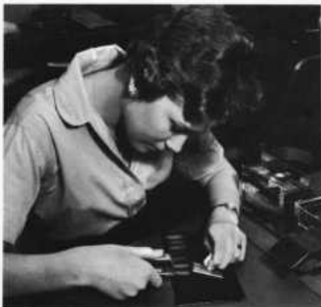
Diane M. Moore, a Department technician, uses a fiber sorter to separate and measure cotton fibers.
