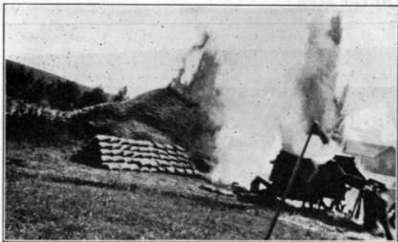
FIG. 107.—Dust explosion in a grain-threshing machine in eastern Washington. These explosions and fires have caused extensive losses to grain and machinery
