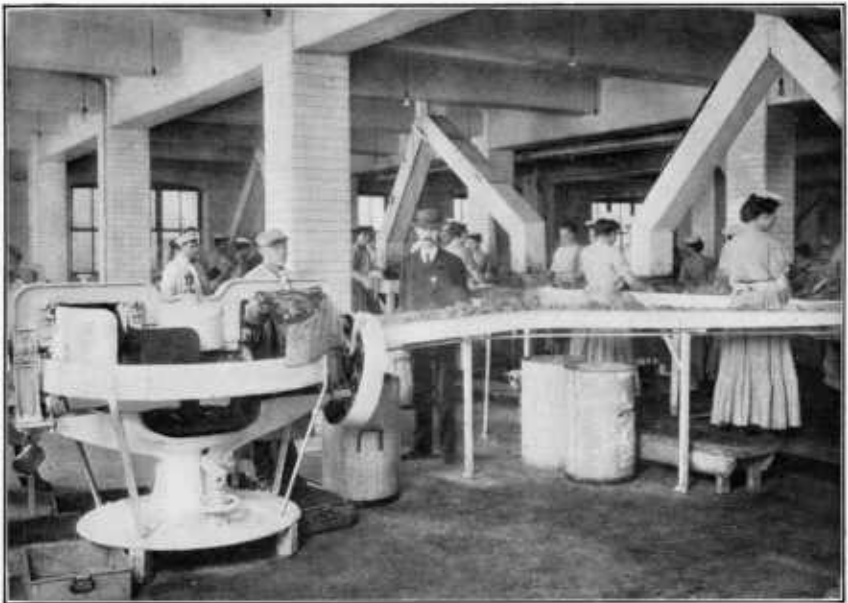
FIG. 2.—PREPARING CORNED BEEF FOR CANNING. [Government inspector at center, Cutting machine shown at left.]
