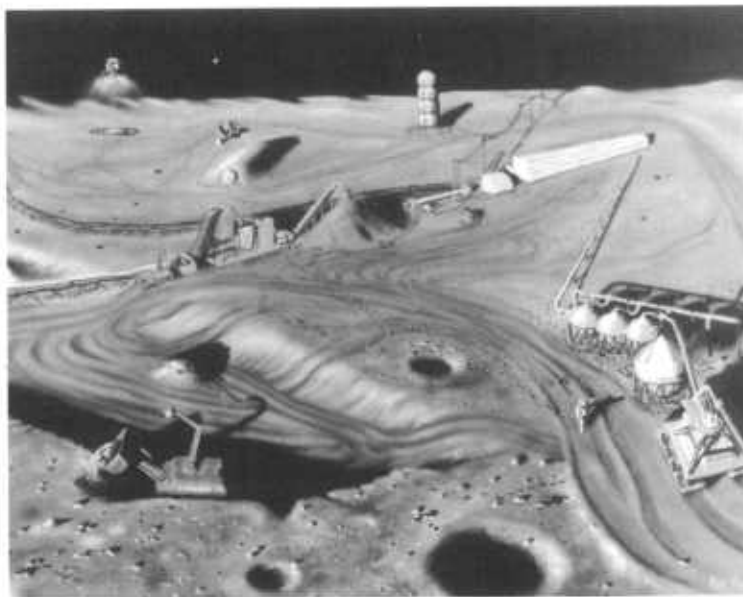
Long-term manned space missions will need basics such as food and air. Artist Pat Rowlings' view of a future lunar mining operation illustrates the production of liquid oxygen. Ilmenite, a fairly common oxygen-rich component of lunar soil, is shown being processed into liquid oxygen that will be used by the orbiting space station.
