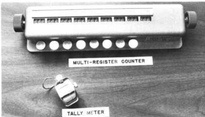
Figure 24 —Multiregister counter and tally meter used in registering counts of budworm larvae and other arthropods.
