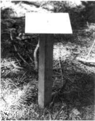
Figure 1 —Field placement of Minnesota trap for measuring early-larval dispersal of jack pine budworm.
