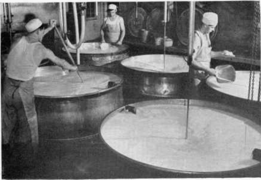
FIGURE 3.—Turning the surface under (background) ; harping the curd (left) ; testing the curd preparatory to dipping (right).
