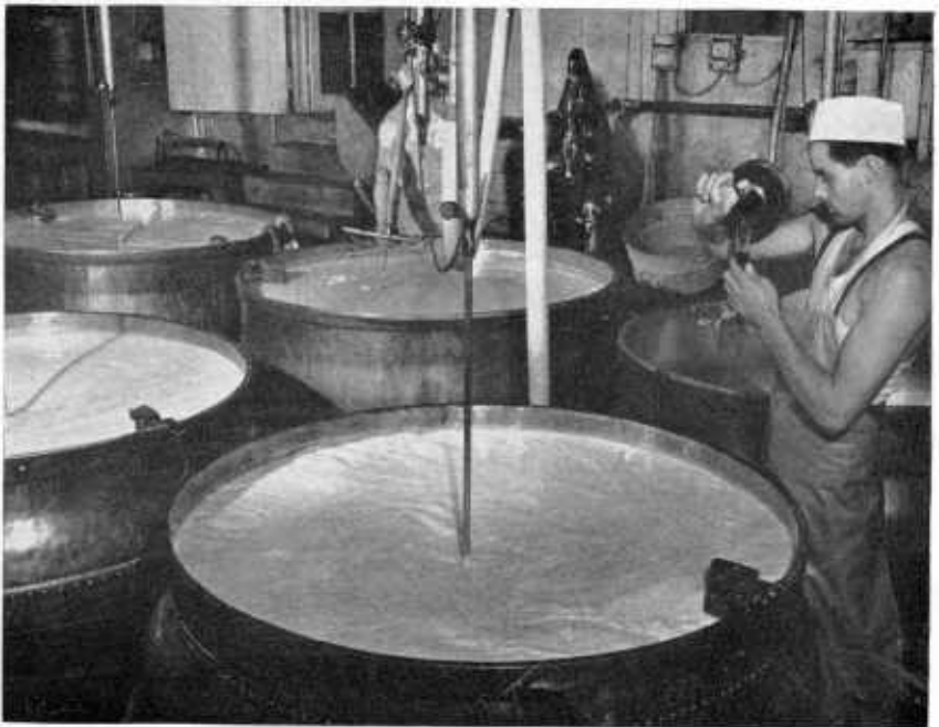
FIGURE 2.—Measuring the rennet (right), which will be diluted with water and added to the milk being stirred in the kettle (foreground); cutting the curd (rear center).
