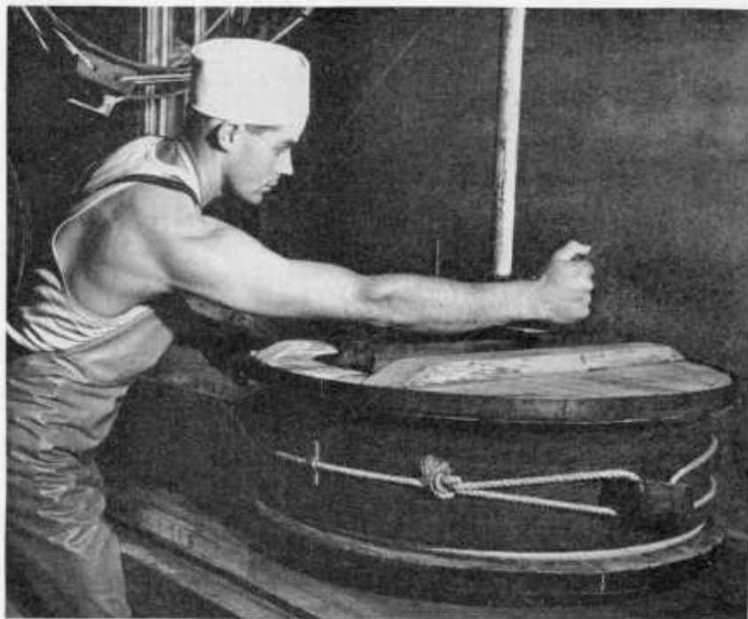
FIGURE 6.—Pressing the curd in the hoop with a screw press suspended from above.
