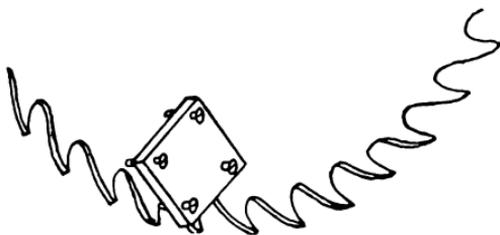
Figure 3.—Side gage for alining saw teeth.
