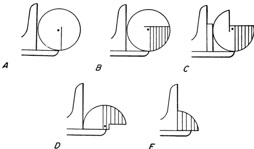
Figure 11.—Steps in sawing oversize logs: *A*, Initial cut; *B*, turned up  $90^\circ$  from *A*, and sawed; *C*, turned  $90^\circ$  from *B*, and sawed; *D*, turned down  $90^\circ$  from *C*, and sawed; *E*, turned down  $90^\circ$  from *D*, and sawed.
