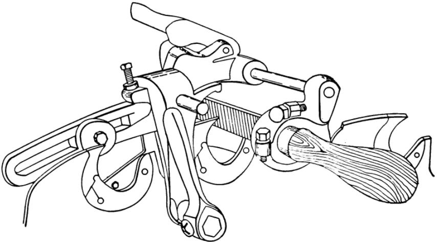
Figure 6.—File in frame for sharpening teeth.
