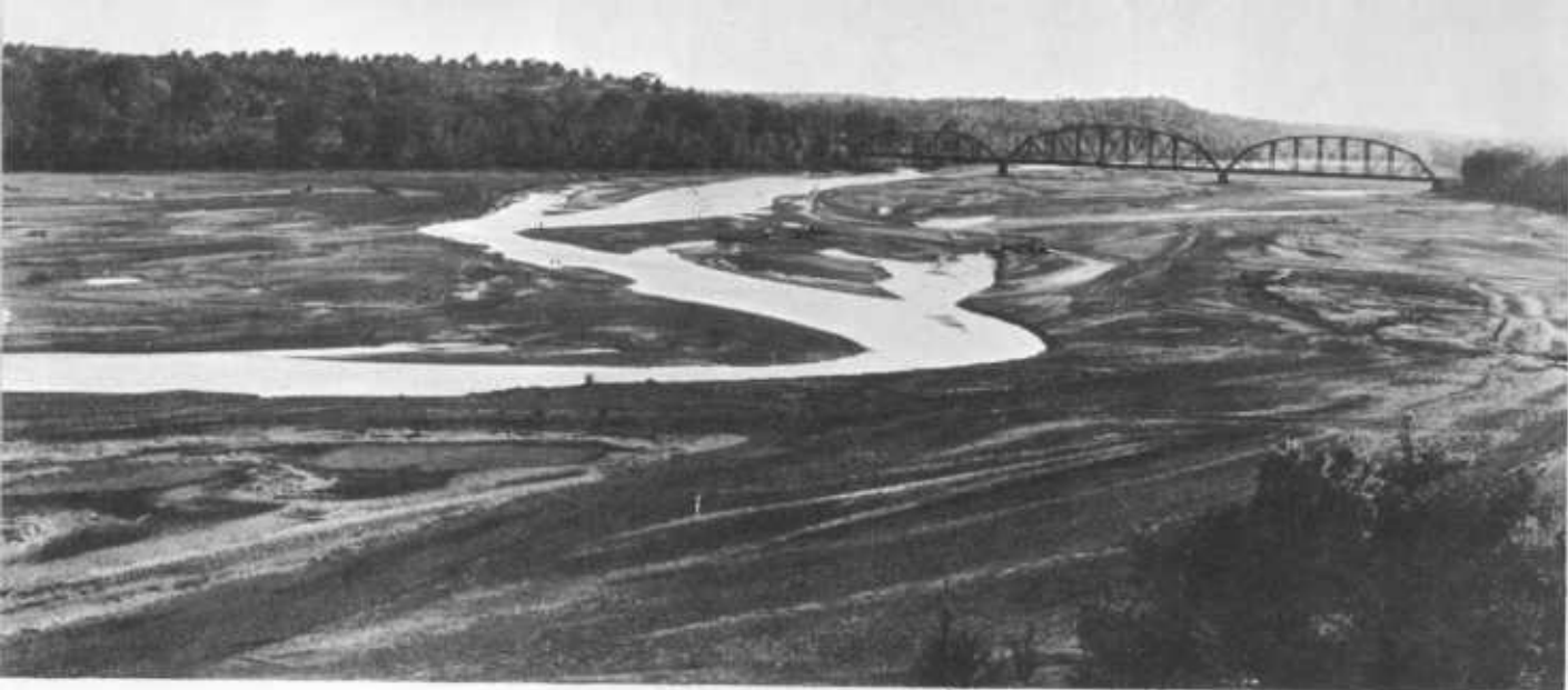
Silted-up channel of Canadian River, Okla. The bridge in the background may soon need to be raised if it is to be useful.
