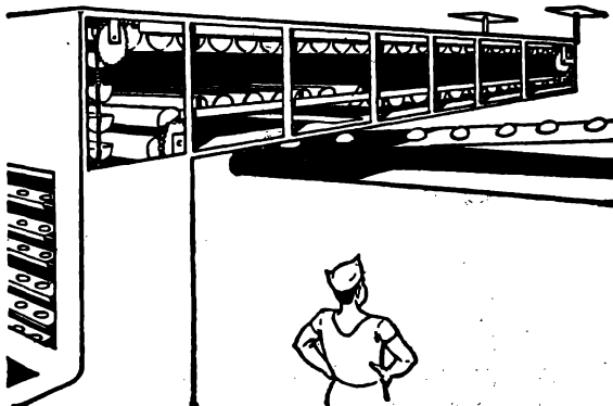
5. The dough "recovers" in the overhead proofer.
