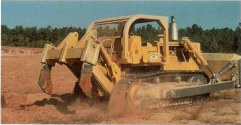
**Figure 10**—Subsoiling is one method of improving compacted soils in the Piedmont.
