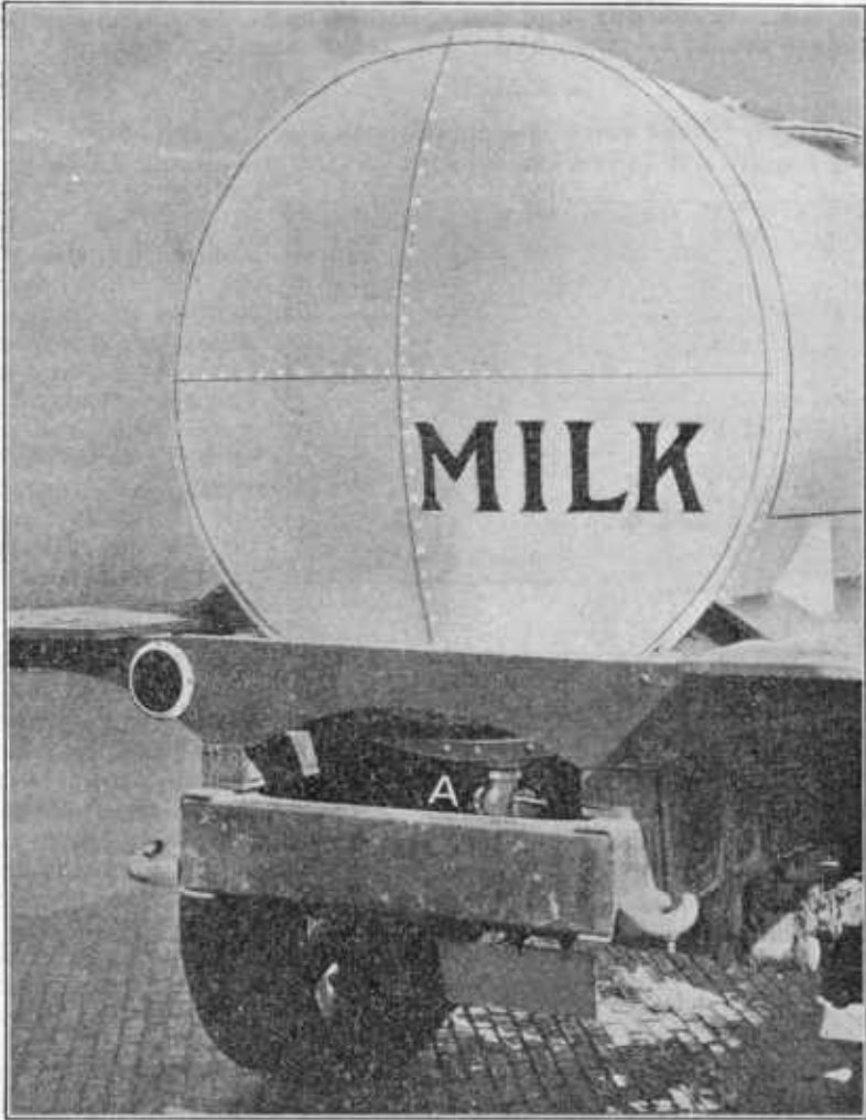
FIGURE 3.—The valve (A) on this milk-tank truck is difficult to reach for cleaning and unloading
