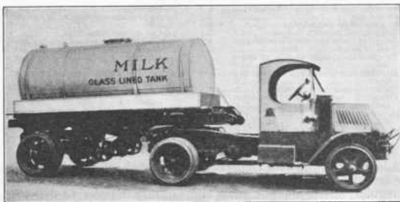
FIGURE 1.—A semitrailer, equipped with air brakes, on which a 2,000-gallon milk tank is mounted
