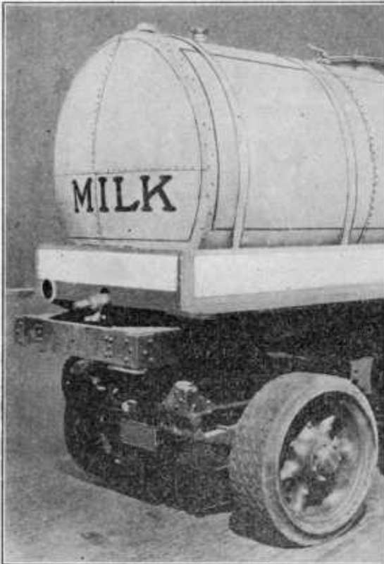
FIGURE 4.—The valve on this milk-tank truck is in an accessible position. Dust cap has been removed
