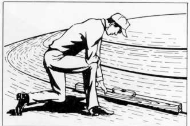
Use carpenter's level mounted on a 2 by 4 to lay out contour line.
