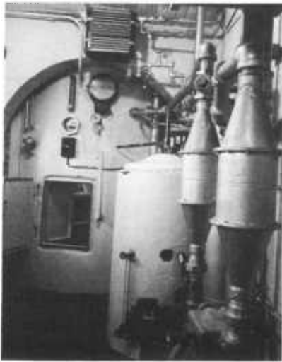
High altitude chamber used for Colorado studies on the effects of atmospheric pressure in food preparation.
