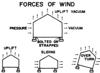
Since wind may lift or slide houses off their foundations, houses must be securely fastened to the foundation.
