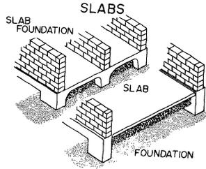
The slab foundation is a special foundation which floats on top of the soil and also serves as the floor of the house. The slab is thickened under all of the walls to support their heavy loads.
