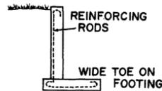
Other jobs of a foundation wall are to insulate and to moisture proof. Basements have been traditionally used as cellars to store foods and supplies, especially in the colder climates. But in recent years, with less need for long term food storage, houses are being built without basements or with basements to be used as family living areas and/or game rooms. If you are going to use your basement as a living area,
