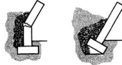
tying the wall to anchors in the soil, or counter-balancing the wall.
