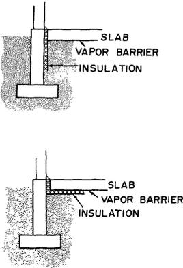
Since concrete is a good heat conductor, you must take special care when concrete slabs are installed close to the soil surface. A sheet of rigid insulation may be installed vertically down the inside of the foundation wall, or between the floor slab and the foundation wall and then horizontally under the slab.
