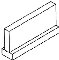
Continuous walls are used to support heavy loads or to enclose a crawl space or basement. If enclosure of space is the main objective, then the wall may be built of lighter, more porous insulating materials which will reduce heat loss and sound transmission.
