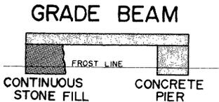
A grade beam foundation is a pressure-treated wood or reinforced concrete beam which is submerged to a depth of about 8 inches below grade. It may be supported on a stone fill or on underground piers which extend into the ground below the frost line.
