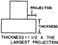
Thickness of the footing depends on how far it protrudes beyond the foundation wall. The rule is that the thickness should be  $1\frac{1}{2}$  times as great as the largest projection.
