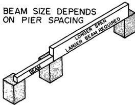
The size of such a beam depends on the load it must carry and the distance between piers. The space between piers is generally enclosed with curtain walls which carry no load and whose main purpose is to enclose the space and act as a barrier to wind, heat, moisture, and sometimes, animals.
