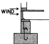
For masonry walls the fastening device should be extended through the foundation to the footing. In all cases there should be a continuous tie extending as far into the soil as practical.
