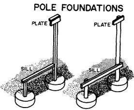
they are made of other materials. The pole or post foundation is a special kind of pier foundation built of pressure-treated wood. It is often used on steep terrain where there is considerable variation in the height of the piers and where a regular masonry pier might bend and break.
