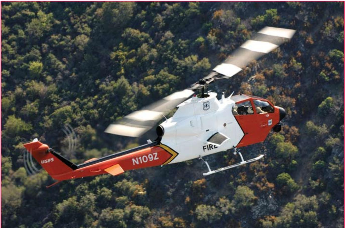
*This former U.S. Army Bell 209 AH-1 helicopter—now known as “Firewatch”—has been specially equipped for experimental use on Pacific Southwest Region fires. This ship boasts everything from sophisticated lasers to real-time video and state-of-the-art remote sensing programs. Photo: courtesy Dan Megna.*
