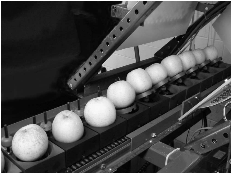
Fig. 3. Conveyor and imaging area. Apples are tilted 45^\circ while they rotate in front of the camera. This is located out of view of the image, outside the upper right hand corner.
