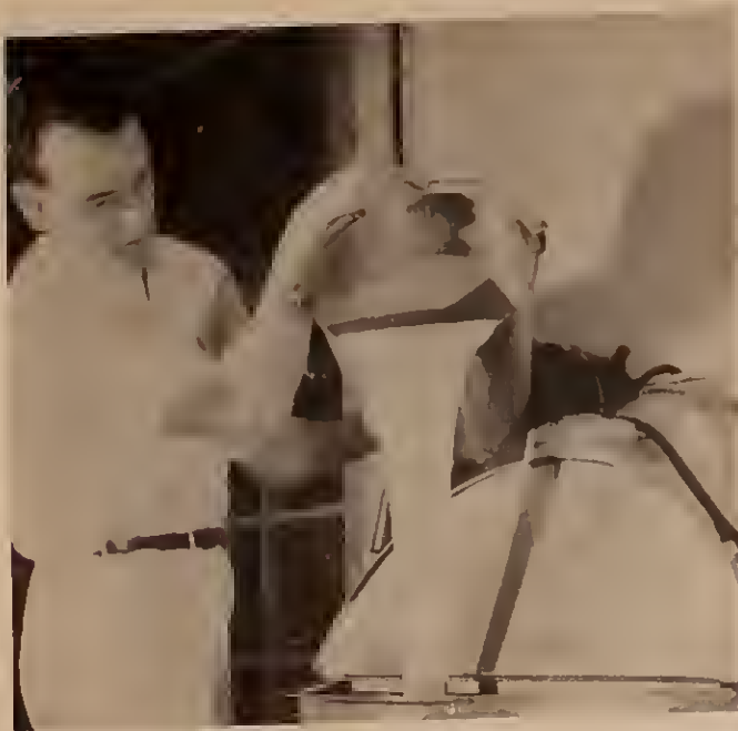
Frank E. Potter, dairy manufacturing technologist, adds sweetened condensed buttermilk to the ice cream "mix" in the pasteurizer. The "mix" is then pasteurized by heating it to 160 degrees F. for half an hour.
