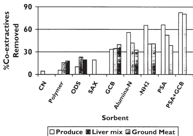
**Figure 5.** Cleanup capabilities of different sorbents using dispersive-SPE of 1 g/mL MeCN extracts of mixed fruit and vegetable samples (lettuce, tomato, apple, strawberry, orange, spinach, grapes, and carrot), mixed liver samples (calf, pork, and chicken), and ground beef in which 1 g NaCl + 4 g MgSO<sub>4</sub> was used to induce partitioning.
