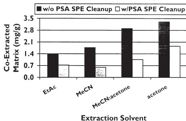
**Figure 1. Comparison of different solvents in extraction of a mixture of fruits and vegetables in the final method with and without dispersive-SPE cleanup step using PSA sorbent. Co-extracted matrix is amount (mg) dissolved in extract vs original sample amount extracted (g). The ratio of MeCN:acetone was 1:1.**
