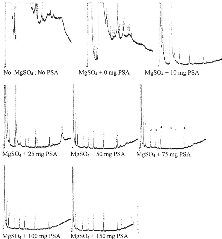
**Figure 6.** GC-FPD analysis of asparagus spiked at 2.0 ng/g using the final method with 5 mL aliquots of extract (equivalent to 5 g sample) evaporated to 1.0 mL and subjected to dispersive SPE cleanup with different amounts of PSA (with or without 150 mg MgSO<sub>4</sub>). Peak identities are methamidophos, acephate, omethoate, dimethoate, chlorpyrifos, and azinphos methyl.
