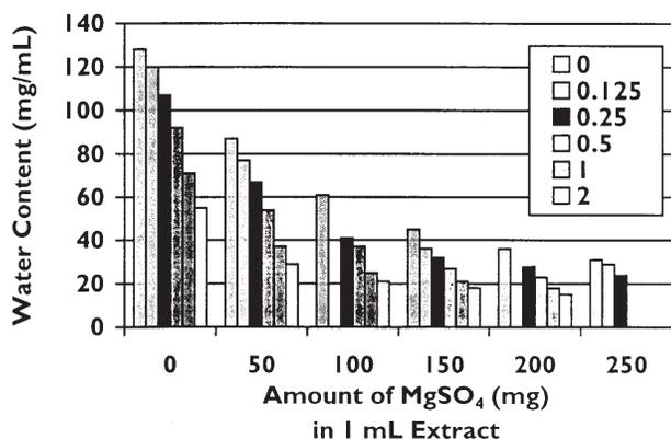
**Figure 4.** Residual water content of apple extracts (1 mL portion of upper layer) dried with different amounts of anhydrous MgSO<sub>4</sub> (NMR used to determine water content). Table legend gives the amount of NaCl used in combination with 5 g MgSO<sub>4</sub> to cause partitioning of 10 g + 10 mL MeCN apple extract.
