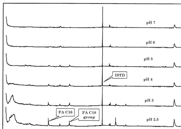
**Figure 3.** Effect of pH on presence of matrix co-extractives in GC/MS (full scan) chromatograms of MeCN apple juice extracts obtained by using 1 g NaCl + 5 g MgSO<sub>4</sub> to induce partitioning. ISTD = internal standard; FA = fatty acid.
