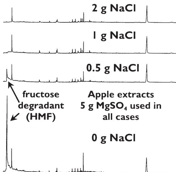
Figure 2. GC/MS chromatograms (full-scan mode) of apple extracts obtained by using different amounts of NaCl with 5 g  $MgSO_4$  in the phase separation between water and MeCN.
