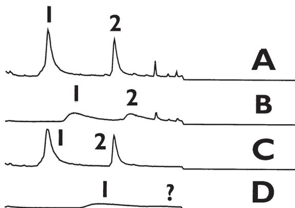
**Figure 7.** Improvement of peak shapes and peak areas with help of 1% ethylglycerol and 500 ppm sorbitol (analyte protectants). GC/MS (SIM) chromatograms of (1) methamidophos and (2) acephate ( $m/z = 94$ ) at the same concentration in A = matrix extracts + analyte protectants; B = matrix extracts; C = solvent + analyte protectants; and D = pesticides in solvent only.
