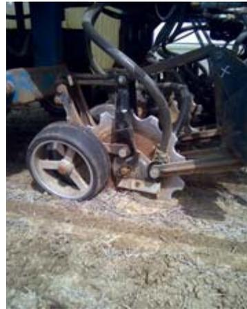
Fig. 3. Cross-slot opener (Cross Slot Inc., Pullman, WA).
