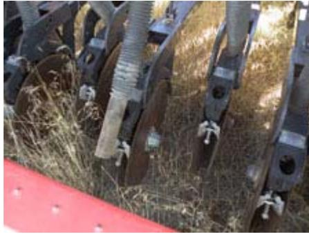
Fig. 1. Conventional double disk openers showing seed tubes attached for drilling seed and unattached for broadcasting seed (International Harvester, Racine, WI, or John Deere, Moline, IL).
