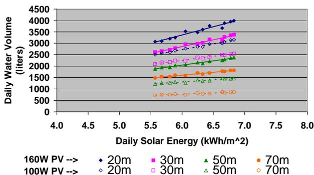
Fig. 16. Measured Shurflo High Head Diaphragm Pump Daily Water Volume.
