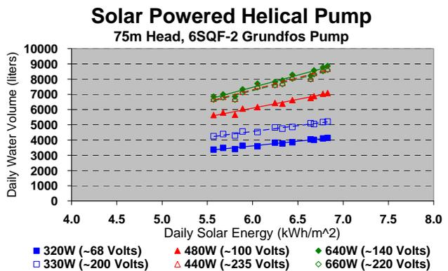
Fig. 11. Affect on Daily Water Volume of Same Type Modules but at Different Voltage Ratings.
