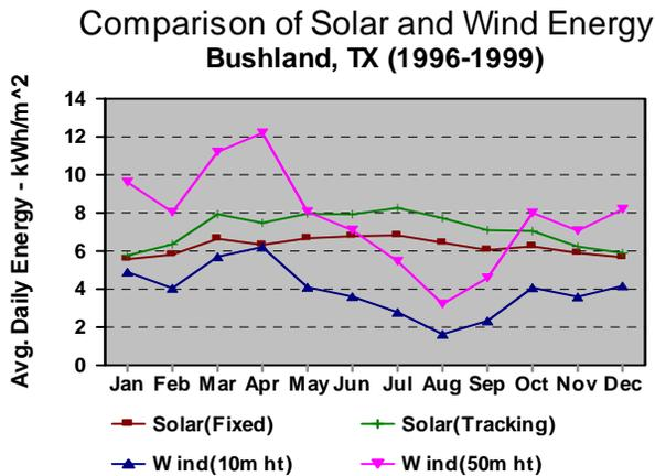
Fig. 6. Comparison of Wind and Solar Energy at Bushland, TX.
