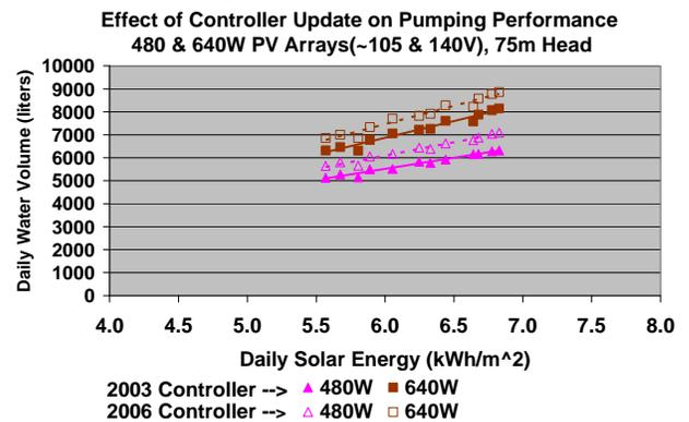
Fig. 14. Effect of Controller Update on Solar Powered Helical Pump System (480 & 640W, 75m Head).
