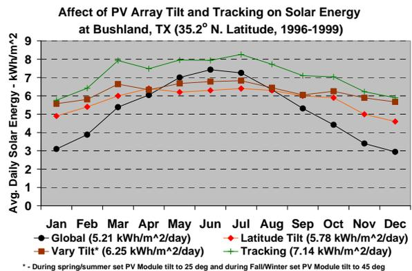
Fig. 9. Measured Daily Solar Radiation at Bushland, TX.
