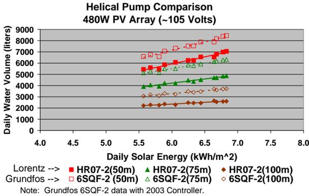
Fig 18. Comparing Daily Water Volume of Two Different Helical Pumps.
