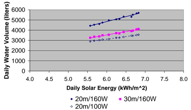
Fig. 17. Measured Sun Pumps Quad Diaphragm Pump Daily Water Volume.
