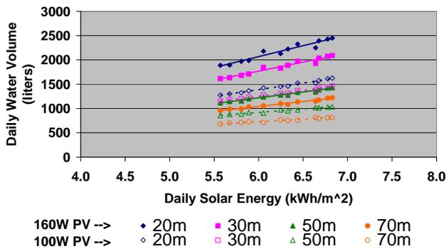
Fig. 15. Measured Sun Pumps High Head Diaphragm Pump Daily Water Volume.
