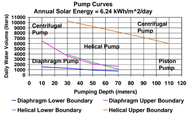
Fig. 20. Determining Type of Pump for Different Daily Water Volume/Pumping Depth Combinations.
