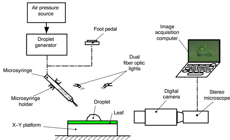
Figure 2. Experimental system to determine contact angle of droplets on waxy leaves.
