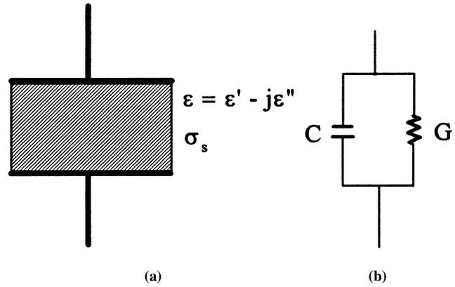
Figure 2—(a) Sample holder of ideal parallel plates; (b) frequency-dependent, measured circuit model, in which C is capacitance and G is conductance.
