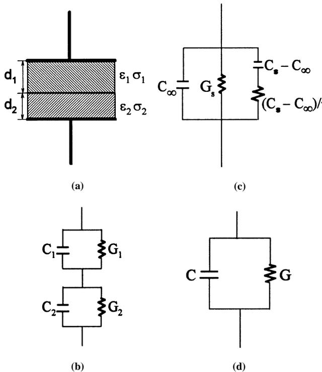
Figure 7—(a) Two-layer heterogeneous system. (b) An equivalent circuit;  $C_1 = \epsilon_0 \epsilon_1 A / d_1$ ;  $G_1 = \sigma_1 A / d_1$ ;  $C_2 = \epsilon_0 \epsilon_2 A / d_2$ ;  $G_2 = \sigma_2 A / d_2$ . (c) Frequency-independent circuit model. (d) Frequency-dependent, measured circuit model.
