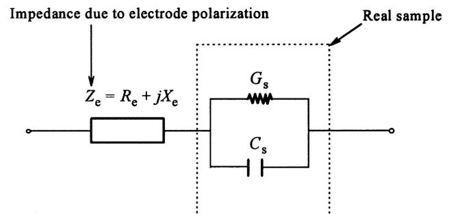
Figure 18—Equivalent circuit for modeling electrode polarization.
