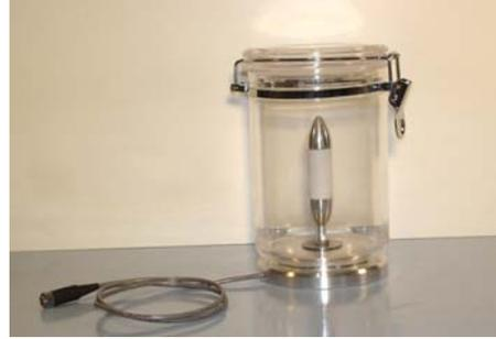
(b) Moisture Sensor Mounted in Canister
