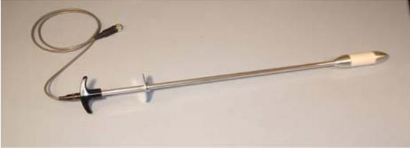
(a) Grain Moisture Sensing Probe
