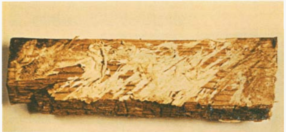
Figure 1 – A decay fungus and its effect on wood. Fungi consist mainly of tiny threads that grow within the wood and can be seen there only with a microscope. In very moist air they may develop on the surface in sufficient quantity to be visible. The upper part of this piece of wood is softened and weakened, and the lower edge is cracked and nearly disintegrated. Decay fungi make no definite galleries like those cut by termites.
