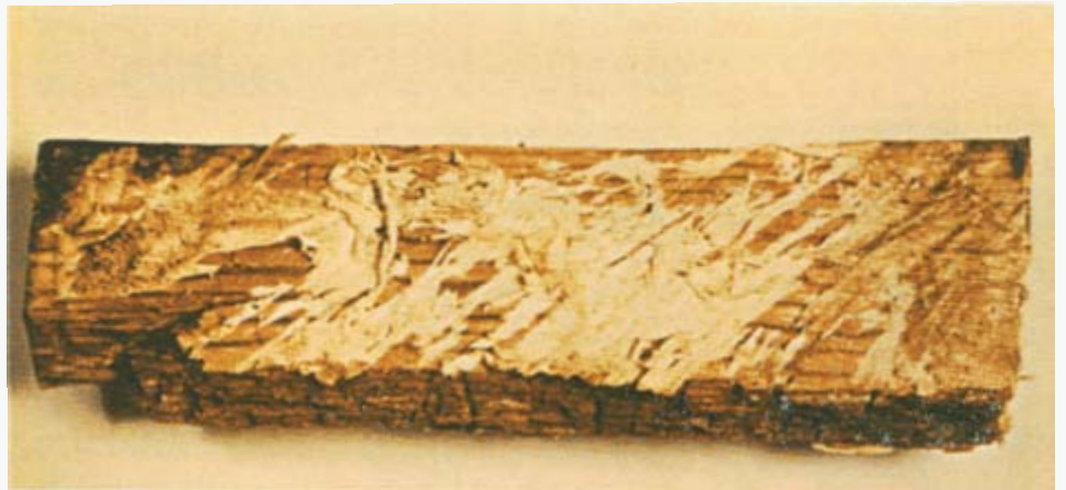
Figure 1 – A decay fungus and its effect on wood. Fungi consist mainly of tiny threads that grow within the wood and can be seen there only with a microscope. In very moist air they may develop on the surface in sufficient quantity to be visible. The upper part of this piece of wood is softened and weakened, and the lower edge is cracked and nearly disintegrated. Decay fungi make no definite galleries like those cut by termites.
