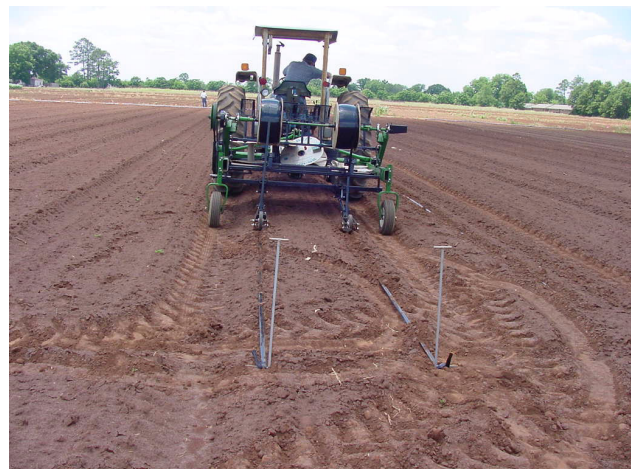
Figure 4. The implement used to install drip tapes in a field with 0.91-m lateral spacing.
