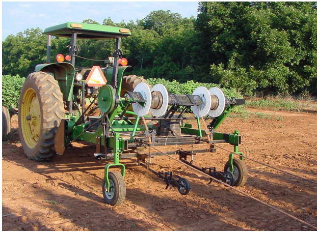
Figure 5. The implement used to retrieve drip tapes in a field with 0.91-m lateral spacing.
