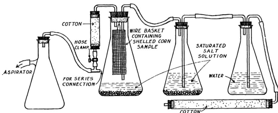
FIGURE 1.—Apparatus used for storing corn under constant-humidity conditions with a slow uniform change of air, and for protecting it from contamination with micro-organisms.
