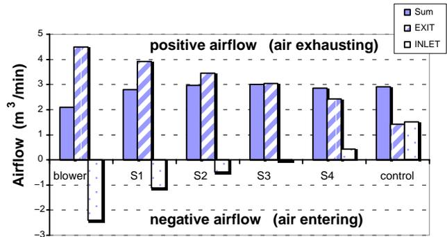
Figure 5. Average inlet and outlet airflow measurements and their summation for corn trials at full grain flow. Spray treatments S1 to S4 are outlined in table 1.
