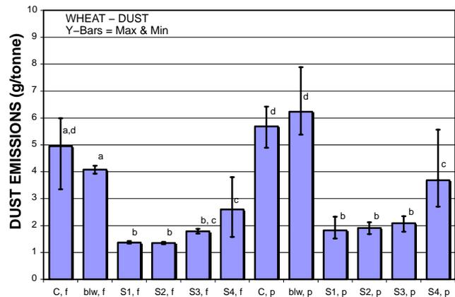
Figure 7. Average, maximum, and minimum dust emissions for wheat at full (f) and partial (p) grain flows. Means with common letter are not significantly different ( $P > 0.05$ ). Spray treatments S1 to S4 are outlined in table 1.
