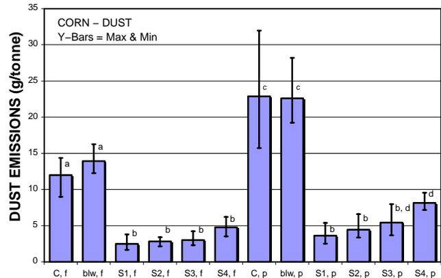
Figure 6. Average, maximum, and minimum dust emissions data for corn at full (f) and partial (p) grain flow. Means with common letter are not significantly different ( $P > 0.05$ ). Spray treatments S1 to S4 are outlined in table 1.
