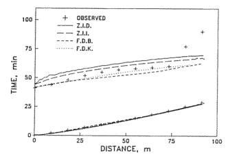
FIG. 6.—Observed Advance and Recession Times for Border AR-15 and Simulated Results Calculated with Z.I.D. and Z.I.I. Models and Full Dynamic Models of Bassett and Fitzsimmons (3), F.D.B., and Katopodes and Strelkoff (12), F.D.K.
