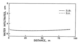
FIG. 5.—Infiltration Depths along Border as Calculated by Z.I.D. and Z.I.I. Models for Border V-5
