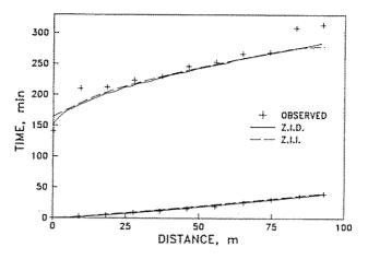
FIG. 3.—Observed Advance and Recession Times for Border V-5 and Simulated Values Calculated with Z.I.D. and Z.I.I. Models
