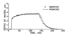
FIG. 4.—Calculated and Observed Ponding Depth versus Time from Start of Irrigation for Point 36.6 m below Head of Border
