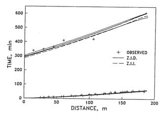
FIG. 2.—Calculated and Observed Advance and Recession Times for McDonnell Farm Border #6. Calculated Curves Are from Model Described in this Paper, Z.I.D., and Zero-Inertia Model Described by Katopodes and Strelkoff (16), Z.I.I. During Recession, Upper Z.I.D. Curve Is for  $\Delta x = 11.6$  m, Lower Curve Is for  $\Delta x = 1.45$  m, and Intermediate Curve Is for  $\Delta x = 1.45$  and 2.9 m
