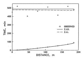
FIG. 7.—Observed Advance and Recession Times for Border CRC-1 and Calculated Values Using Models Z.I.D. and Z.I.I.
