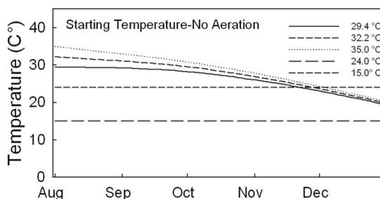
Fig. 1. Predicted temperature of rough rice stored in Beaumont, TX from 1 August to 31 December, with starting grain temperatures of 29.4, 32.2, and 35.0°C. The dimensions of the storage bin were set at 7.7 m in height and 5.5 m in diameter, which can hold ≈10 metric tons of rough rice. The dashed line at 24.0°C represents the approximate lower limit for maximum population growth of stored grain insects; the dashed line at 15°C represents the approximate lower developmental limit.
