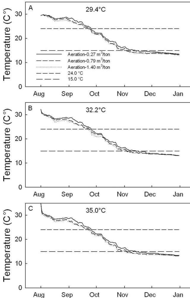
Fig. 3. Predicted temperature of aerated of rough rice stored in Beaumont, TX, from 1 August to 31 December, with starting grain temperatures of 29.4 (A), 32.2 (B), and 35.0°C (C). Storage time, bin dimensions, capacity, and starting insect populations were as described for Figs. 1 and 2; aeration airflow rates were 0.27, 0.79, and 1.4 m<sup>3</sup>/min/metric ton.
