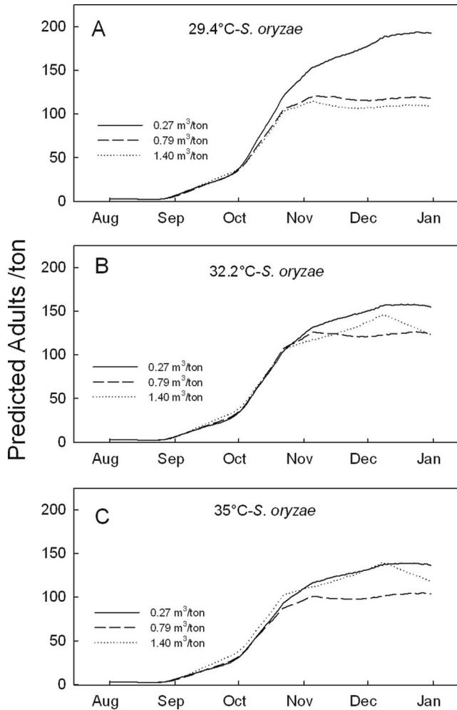
Fig. 5. Predicted populations of adult *S. oryzae* in aerated rough rice stored in Beaumont, TX, from 1 August to 31 December, with starting grain temperatures of 29.4 (A), 32.2 (B), and 35.0°C (C). Storage time, bin dimensions, capacity, starting insect populations, and aeration airflow rates were as described for Figs. 1–4.
