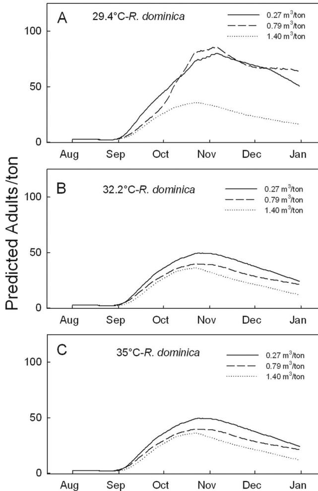
Fig. 4. Predicted populations of adult *R. dominica* in aerated rough rice stored in Beaumont, TX, from 1 August to 31 December, with starting grain temperatures of 29.4 (A), 32.2 (B), and 35.0°C (C). Storage time, bin dimensions, capacity, starting insect populations, and aeration airflow rates were as described for Figs. 1–3.
