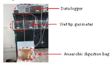
Figure 1. Photo of dry anaerobic digestion system
