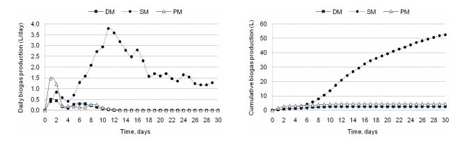
Figure 2. Average daily and cumulative biogas production.
