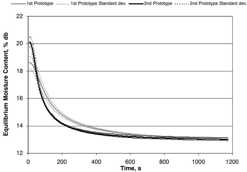
Figure 6. Measurements comparison between the first and second prototype instruments. The sensor probe was approximately 9°C, prior to measurement, and the grain temperature was 21°C.
