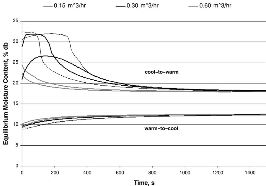
Figure 3. Measured EMC values vs. time for different airflow rates. Two replicates are shown for each airflow. The instrument was transitioning from a cool to warm or warm to cool grain.
