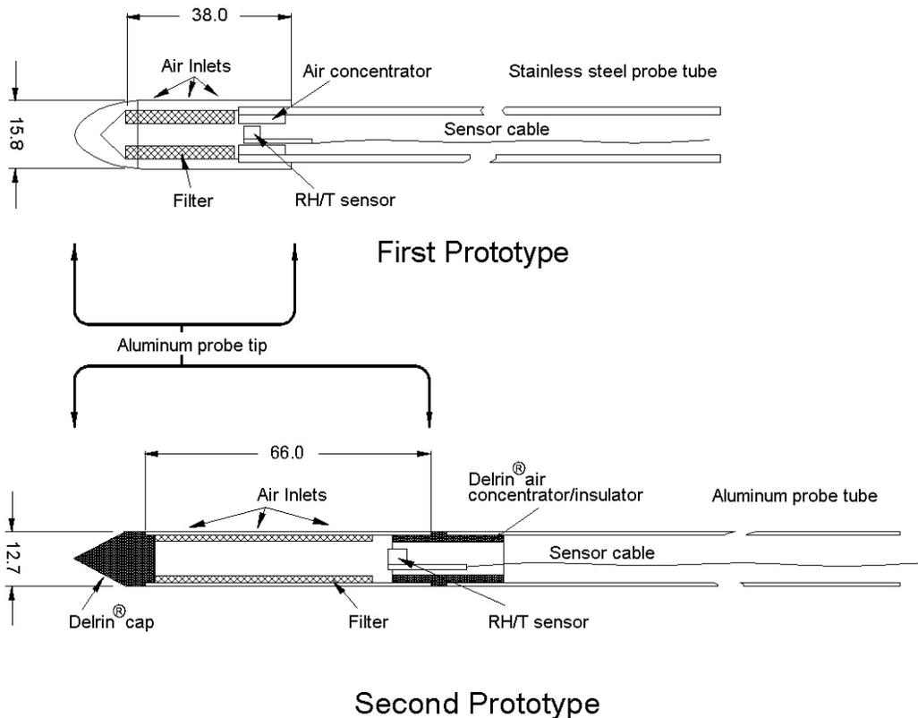
Figure 1. First and second prototypes instruments for EMC measurement (dimensions are in mm).
