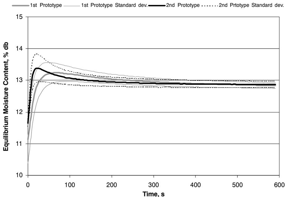
Figure 7. Measurements comparison between the first and second prototype instruments. The sensor probe was approximately 19°C prior to measurement and the grain temperature was 21°C, respectively.
