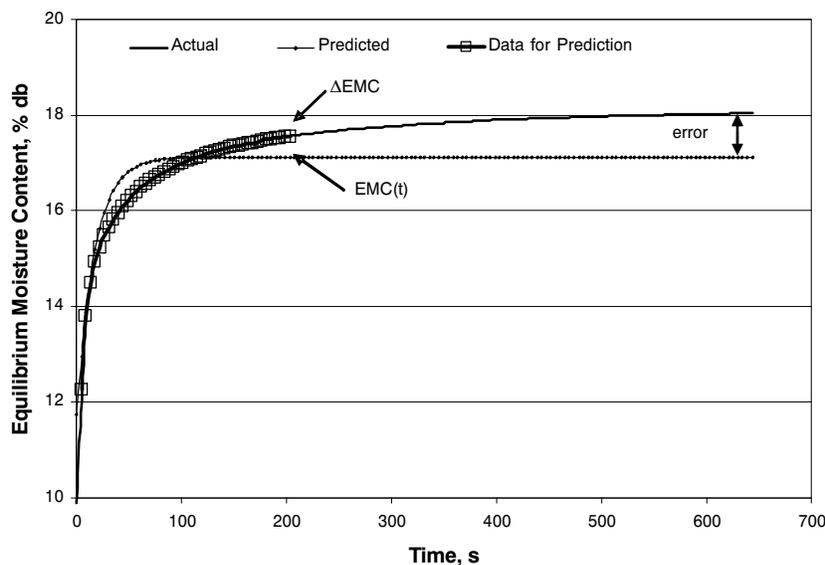
Figure 5. Modeled response of instrument using equation 2 from the first 200 s of data and actual response.
