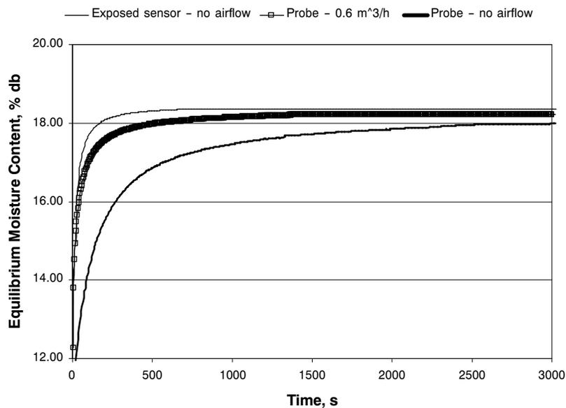
**Figure 2. EMC values vs. time for the first prototype with no airflow, 0.60 m<sup>3</sup>/h airflow and for an exposed sensor.**
