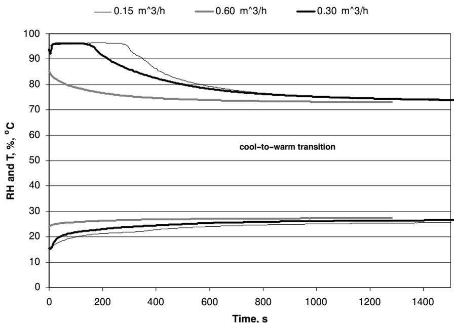
Figure 4. Measured RH and T used to predict EMC values in figure 3 for lower airflows with the instrument transitioning from cool to warm grain for replicate 1.
