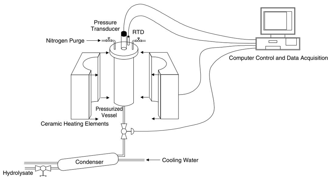
Figure 1. Schematic diagram of pressurized hot water hydrolysis system.
