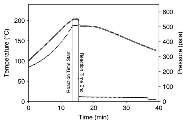
**Figure 2.** Temperature and pressure profile for a typical hydrolysis experiment. For this particular experiment the reaction time was 2 min and the set point temperature was 200 °C.
