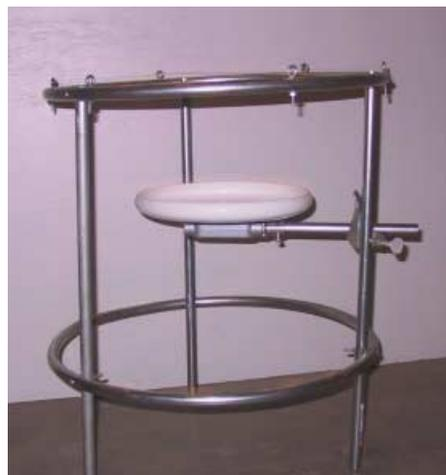
**Figure 3.** One of 12 flying-disk sediment samplers that were mounted in a framework used to adjust sampler height as vegetation height increased. This figure is available in colour online at [www.interscience.wiley.com/journal/esp](http://www.interscience.wiley.com/journal/esp)
