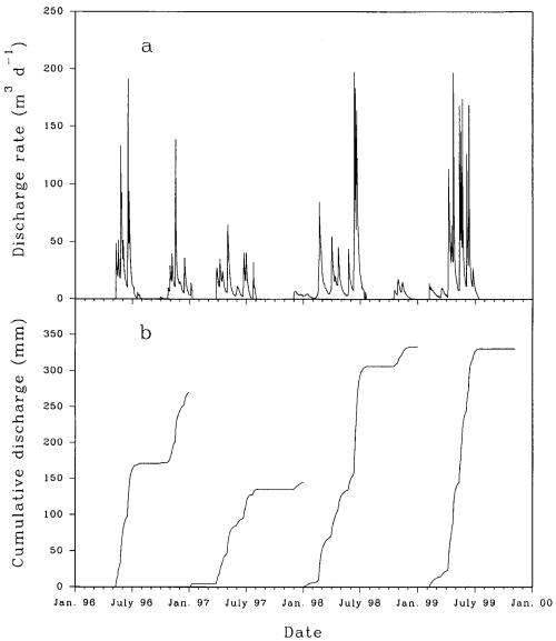
Fig. 3. Example of water discharge rate and cumulative discharge depth from a tile drain for one of the medium (M) nitrogen fertilizer treatment plots for 1996 to 1999.
