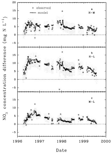
Fig. 5. Observed and modeled differences between mean NO<sub>3</sub> concentrations in tile drainage from plots receiving high (H), medium, (M), and low (L) nitrogen fertilizer treatments starting in spring 1996. Shaded area represents the 95% confidence limits of the modeled NO<sub>3</sub> differences.
