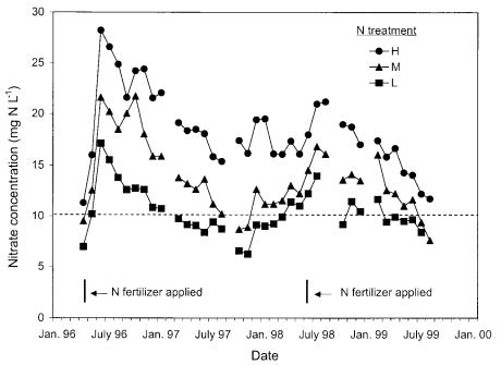
Fig. 4. Nitrate concentrations in tile drains averaged by month and N fertilizer treatment versus time from 1996 through 1999.
