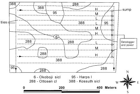
Fig. 1. Schematic of the field showing layout of tile drains, sumps, locations of high (H), medium (M), and low (L) nitrogen fertilizer treatment plots, and distribution of Okoboji silty clay loam, Harps loam, Ottosen clay loam, and Kossuth silty clay loam soils as determined by Brevik et al. (2001).
